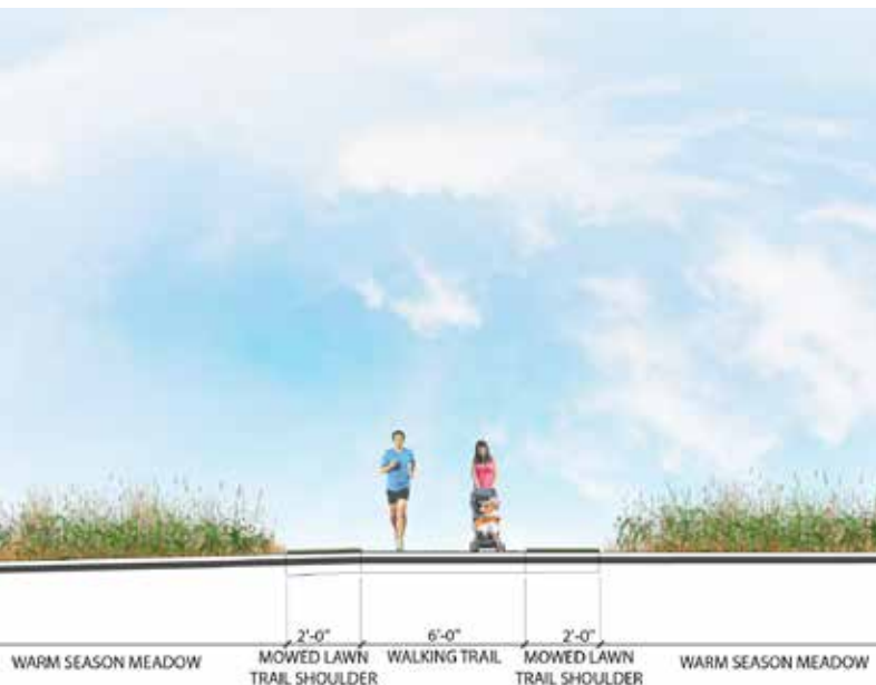
Typical section of the ADA accessible pathway around the Airstrip Meadow.
