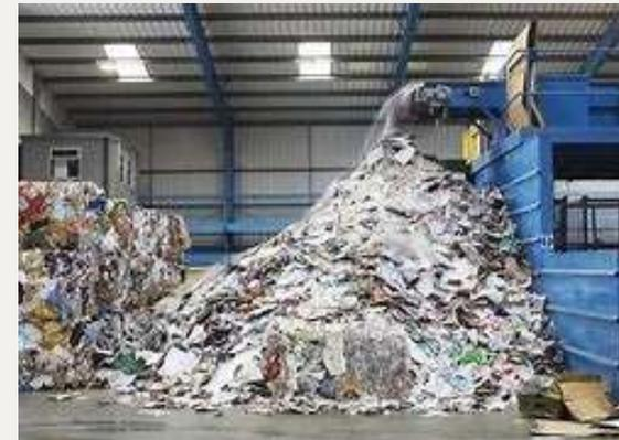
Wish-cycling can also damage expensive processing equipment, such as when plastic bags end up tangled in sorting screens and conveyor belts.
